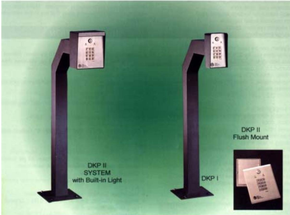
The DKP I's offer solutions to applications requiring access control keypads to control a single entrance or restricted area. The DKP I's may be ordered in either 3 or 4 digit passcode lengths with memory capacities of 1000 and 10,000 codes respectively. They have programmable lockout and door open time, an auxiliary alarm input, and an output for hostage or tamper alarm.
